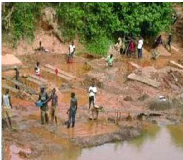
Figure 1(a and b): Showing Unlicensed Miner Washing Tailings Direct Into The River
