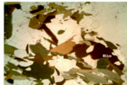
Plate 3: Petrography of Granite Gneiss under Plane and Cross Polar
