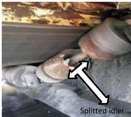
Figure 5a: Tear in a belt due to damaged idler. Figure 5b: Worn out idler due to rusting and friction.
