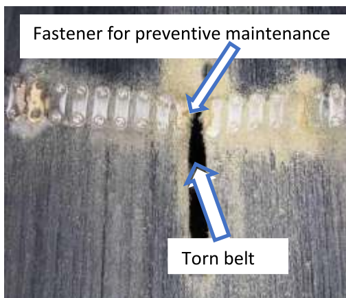
Figure 5c: Aged belt due to abrasive action. Figure 5d: Belt failing across the repaired regions.
