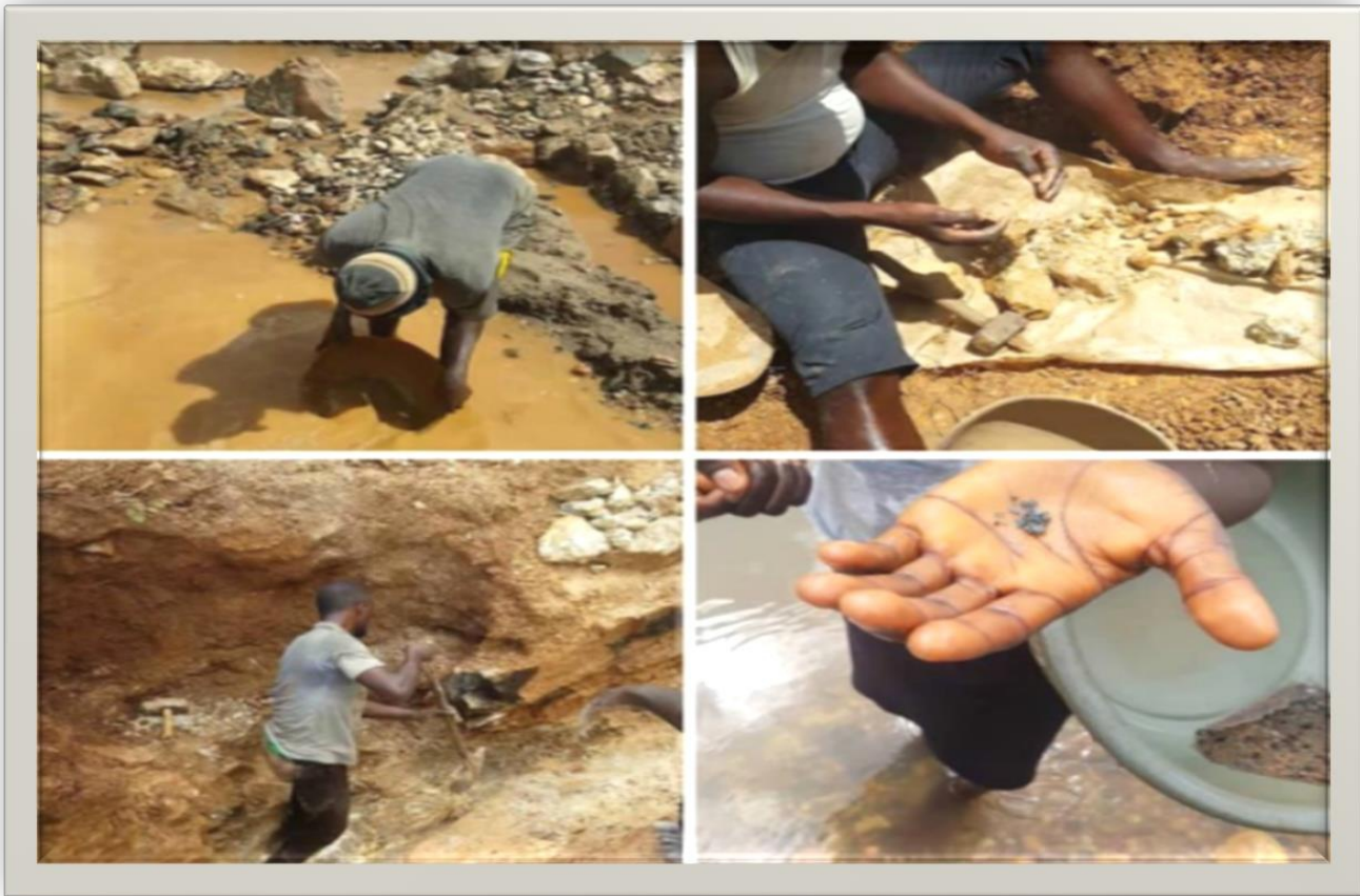
Figure 3.0 Processes involved in the extraction of gemstone: (a) shows an artisanal miner in the process of exploiting gemstone in sediments within the mining site (b) an artisanal miner sorting the gems from the rubble (c) some gems shown off (d) breaking off of rocks containing gems.
